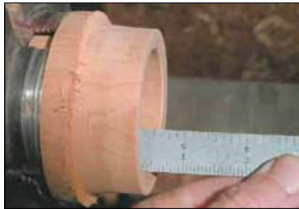
With a 6" ruler, line up the mortise shoulder with the ways. Your goal: a parallel cut or slight outside cant.
