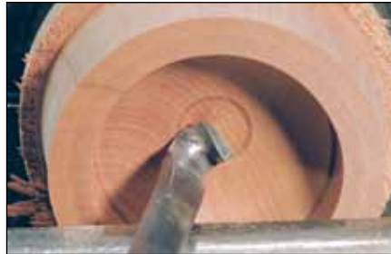
Inside the lid, the hook tool performs two actions: working with the grain and cutting the wood.
