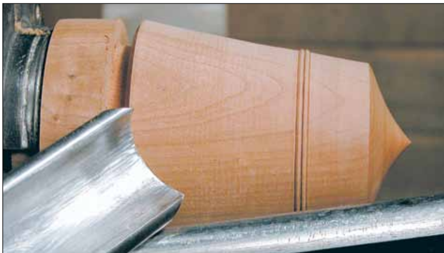
Complete the outer side of the box with a roughing gouge. Add fine detailing at the joint or the top of the lid with a skew chisel or detail gouge.
